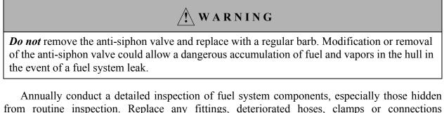
immediately. Fuel filter/water separators should be replaced at least annually.
