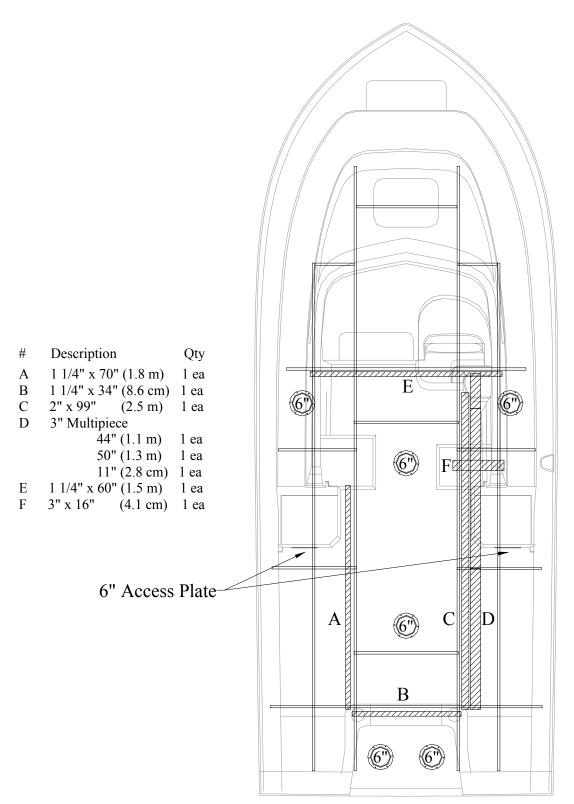
Access Plate And Rigging Tube Locations
