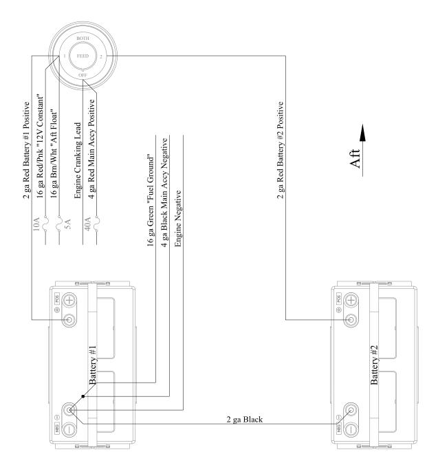
Battery Wiring with Select Switch
